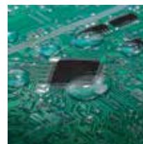
Water-Resistant Printed Circuit Board (PCB)
