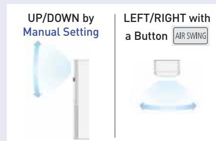
S-34/43/48PB3Q6 Blow distance: Up to 11 m
